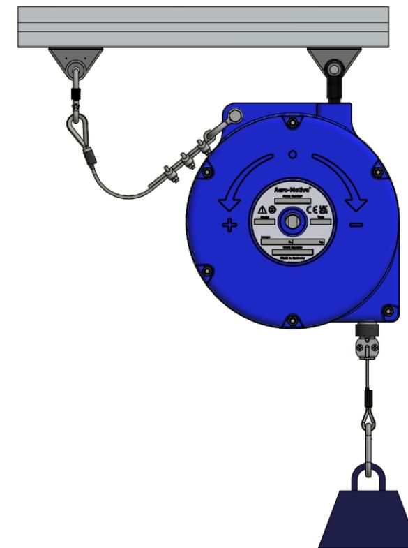
\*- SECONDARY SUPPORT CABLE SHOULD BE AS SHORT AS POSSIBLE,
